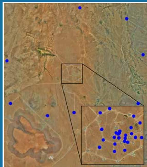
The 32 AR1.5 antennas include 24 in the core and 8 on "long baselines" (located approximately on a circle about 4 kilometres from the core). These 32 positions are indicated by the collection of blue dots. The square box, showing a zoomed-in version of the core of the MeerKAT array, is 1.2 kilometres on the side.
