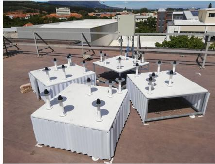
**Figure 1 – The 24-element transient array radio telescope at Stellenbosch University**
