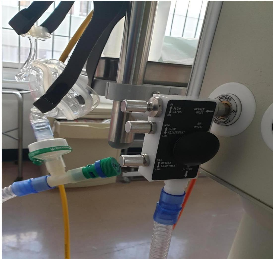
**Illustration 4:** The UCL VENTURA air/oxygen blender plugged directly into a standard hospital oxygen supply port and providing gas to a half-face mask CPAP patient circuit via a 22 mm flexible tube
