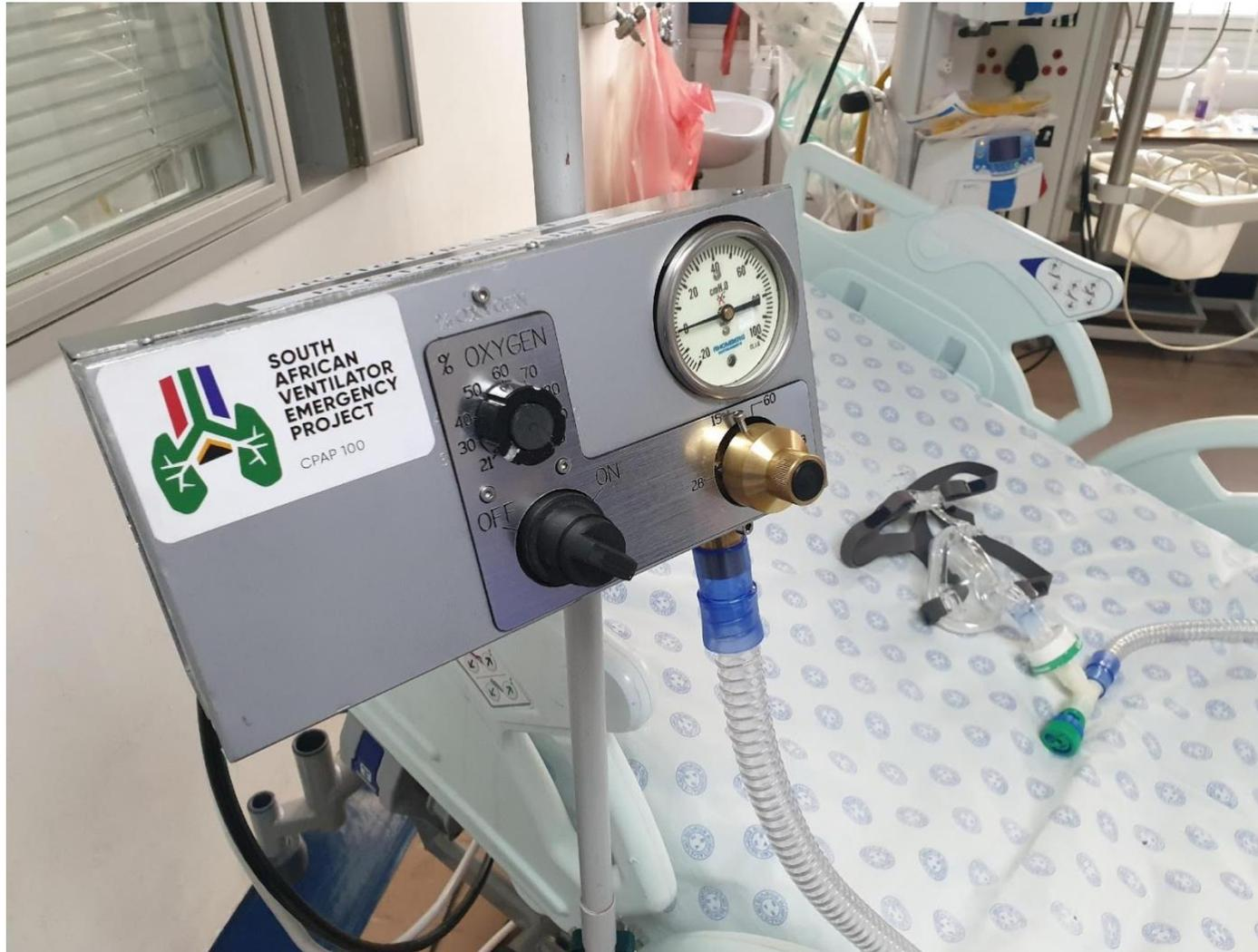
**Illustration 2:** The SAVE-P air/oxygen blender connected to standard hospital oxygen and medical air supply ports via colour-coded hoses and providing gas to a half-face mask CPAP patient circuit via a 22 mm flexible tube.
