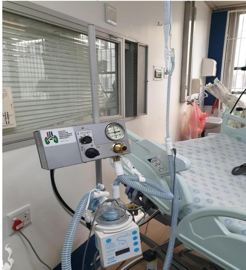
**Illustration I:** The SAVE-P air/oxygen blender providing gas for a HFNO system. The blender outlet connects directly to a standard humidifier, which provides heated and humidified gas to the high-flow cannula.
