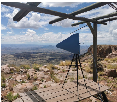
RFI testing at a candidate AMT site in Namibia.
