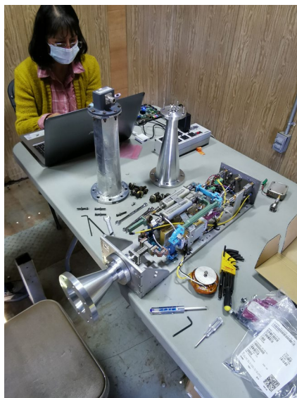
PhD student programming an FPGA Spectrometer for the K-band receiver, Tulancingo, México.
